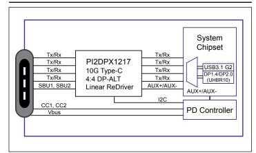
System with USB Type-C Connector Application
