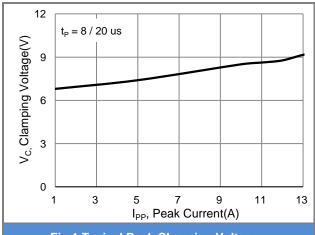
Fig.1 Typical Peak Clamping Voltage
