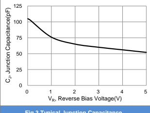
Fig.3 Typical Junction Capacitance
