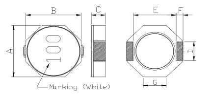
A: 8.00±0.3 mm B: 8.00±0.3 mm C: 4.50 Max mm D: 2.50 Typ. mm E: 6.30 Typ. mm F: 1.20 Typ. mm G: 3.30 Typ. mm
