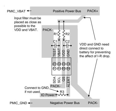
Figure 9. PCB Layout Guide
