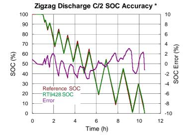
\*: Sample accuracy with custom parameters into the IC.
