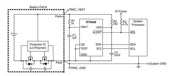
Figure 6. RT9428 Application Example with Alert Interrupt
