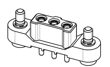
SPECIFICATIONS: MATERIAL: HOUSING = GLASS-FILLED PA46 UL94V-0, GREEN CONTACT CLIP = BERYLLIUM COPPER CONTACT SHELL = BRASS JACKSCREW, CIRCLIP = STAINLESS STEEL FINISH (ALL OVER NICKEL): 0.10/0.17μm GOLD CLIP, 0.25/0.30μm GOLD SHELL PACKING: FOR COMPLETE SPECIFICATION, SEE COMPONENT SPECIFICATION CO48XX (LATEST ISSUE)
