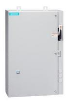
Non-reversing motor starter, Size 2, Three phase full voltage, Solid-state overload relay, OLR amp range 13-52A, 24VAC 50-60Hz coil, Combination type, 60A fusible disconnect, 60A/250V fuse clip, Enclosure NEMA type 4/12, Water/dust tight for outdoors, Extra-wide enclosure
