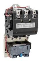
Non-reversing motor starter Size 3 Three phase full voltage Solid-state overload relay OLRelay amp range 25-100A 190-220/220-240V 50/60HZ coil Combination type No enclosure
