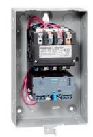
Non-reversing motor starter, Size 1 3/4, Three phase full voltage, Solidstate overload relay, OLR amp range 10-40A, 240V 50Hz / 277V 60Hz coil, Non-combination type, Enclosure type 1, Indoor general purpose use, Standard width enclosure
