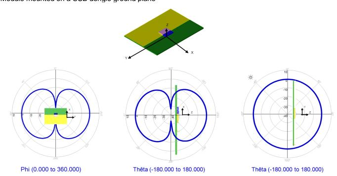
Gain measurement in dBi @ 2.45 GHz.
