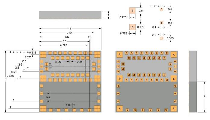
Dimensions in mm Tolerance: +/- 0.03 mm
