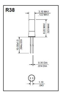
NOTE: Through hole device can withstand 245°C soldering by terminals only
