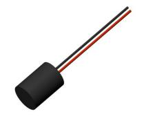
**A240A** works as a signal transmitting and receiving unit. This ultrasonic transducer is suitable for non-contact level detection and proximity measurement with extraordinary reliability. In particular, the transducer with the PVDF housing can operate under harsh chemical environment to measure the level of fluids, pastes, and coarse bulk materials.
