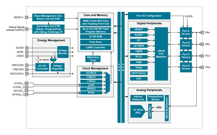
Figure 3.1. Detailed EFM32PG22 Block Diagram
