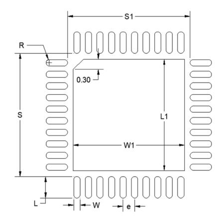
Figure 8.2. QFN40 PCB Land Pattern Drawing
