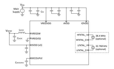
Figure 5.2. EFM32PG22 Typical Application Circuit: DCDC Configuration, AVDD and IOVDD from main supply
