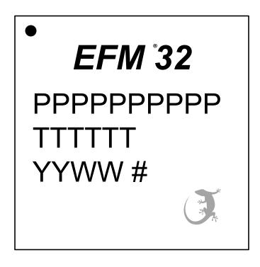
Figure 8.3. QFN40 Package Marking
