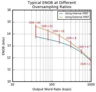
Figure 4.10. Typical ENOB vs. Oversampling Ratio
