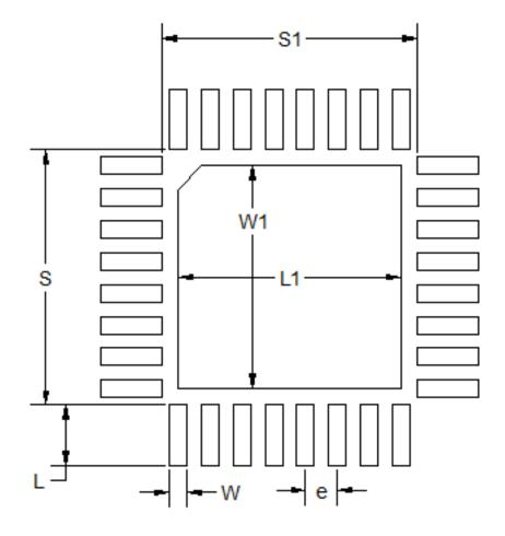
Figure 7.2. QFN32 PCB Land Pattern Drawing
