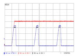
Since both Vo1 and Vo2 have the same delay and slew rate settings they will continue to turn off and on synchronously every 130ms as shown in Figure 37 until the condition causing the undervoltage is removed.
