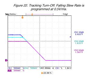
Figure 23. Turn-Off with Tracking and Sequencing. Falling Slew Rate is programmed at 0.5V/ms.
