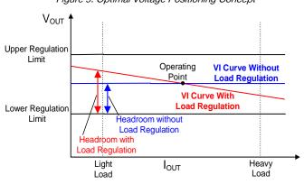
Figure 9. Optimal Voltage Positioning Concept
