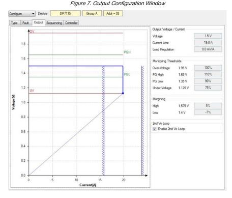
Note that the GUI shows the effect of setting PG, OV and UV limits as both values and graphical limit bars. Vertical hashed lines are error bars for the Overcurrent (OC) limit.
