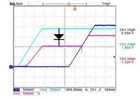
Figure 21. Turn On into Prebiased Load. V3 is Prebiased by V2 via a Diode.
