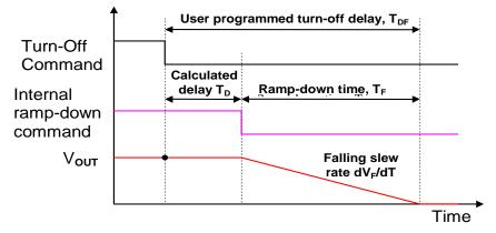
As it can be seen from Figure 16, the internally calculated delay  $T_D$  is determined by the equation below.
