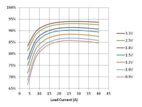
Figure 3. Efficiency vs Load, Vin=8V, Fsw=500KHz
