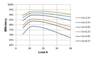
Figure 5. Efficiency vs Vout, Load=40A, Fsw=500KHz
