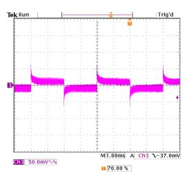
Figure 45. Transient Response with Regulation set to 0.55mV/A
