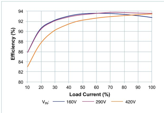
Figure 10 —  $V_{IN}$  to  $V_{OUT}$  efficiency,  $T_{CASE} = -40^\circ\text{C}$
