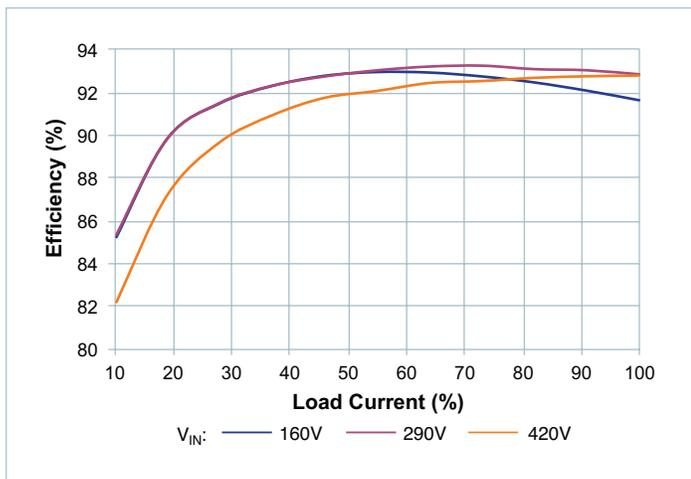
Figure 12 —  $V_{IN}$  to  $V_{OUT}$  efficiency,  $T_{CASE} = 25^\circ\text{C}$
