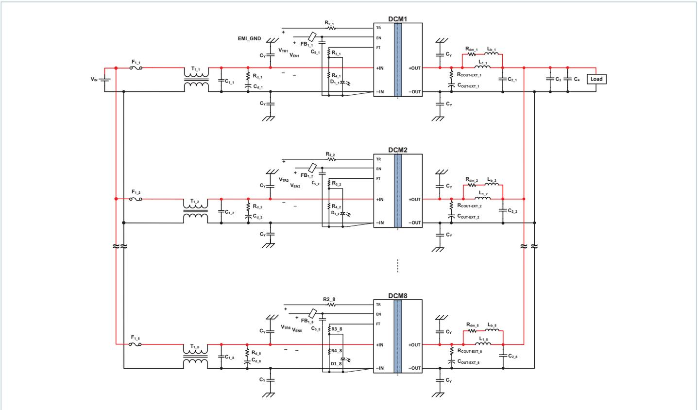
Figure 26 — DCM paralleling configuration circuit 2
