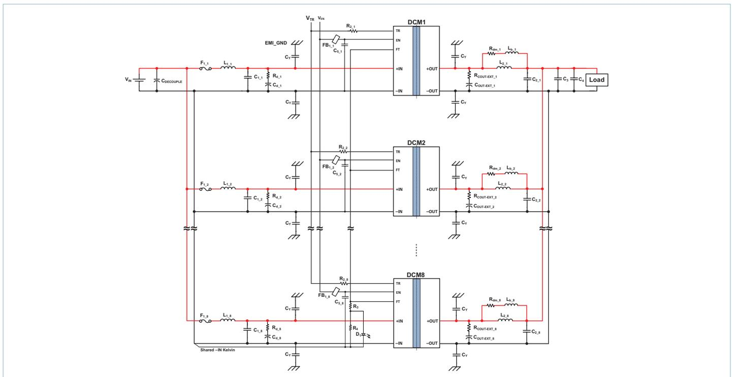
Figure 25 — DCM paralleling configuration circuit 1
