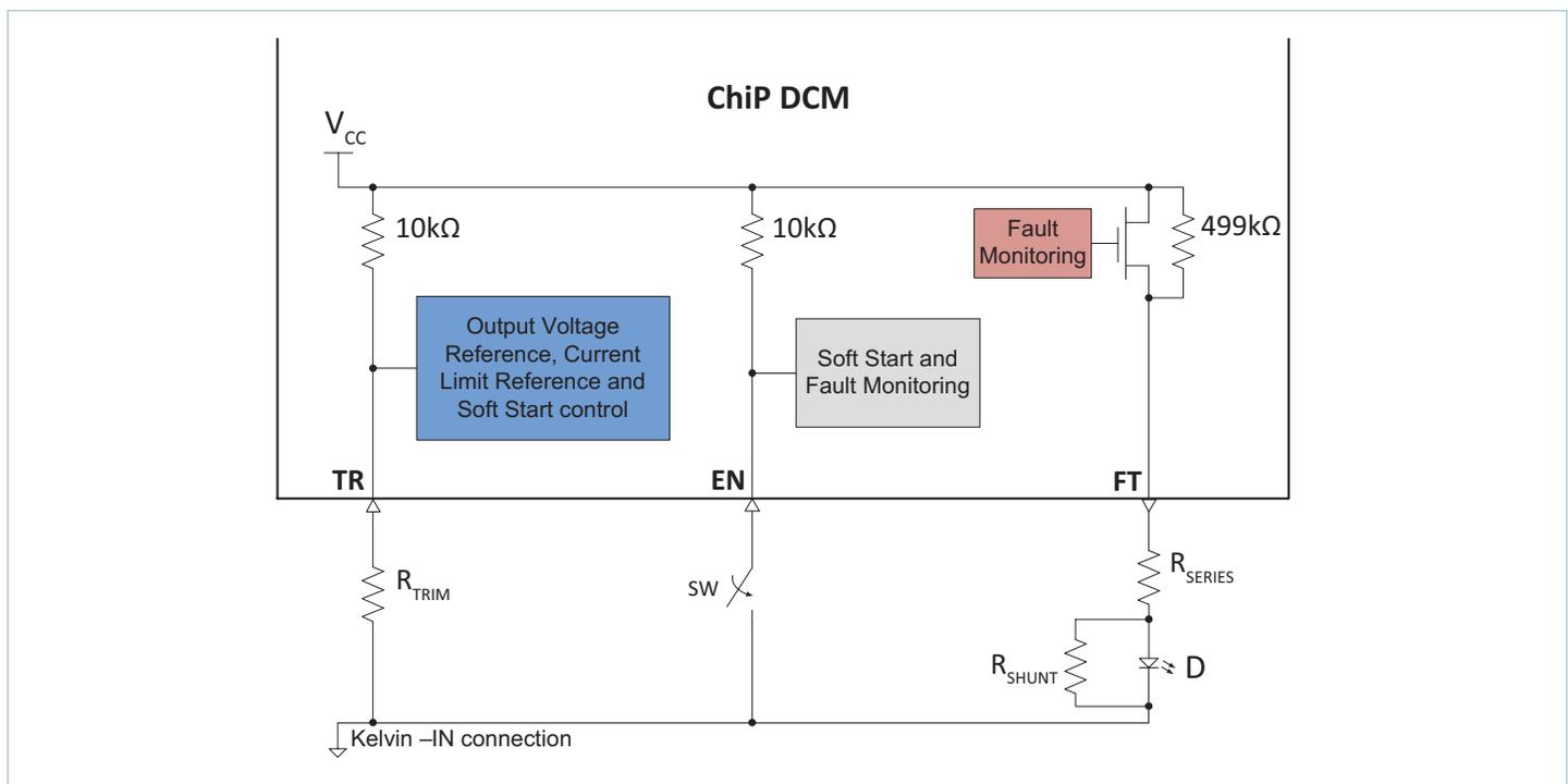
The DCM will latch trim behavior at application of  $V_{IN}$ , and persist in that same behavior until loss of input voltage.
