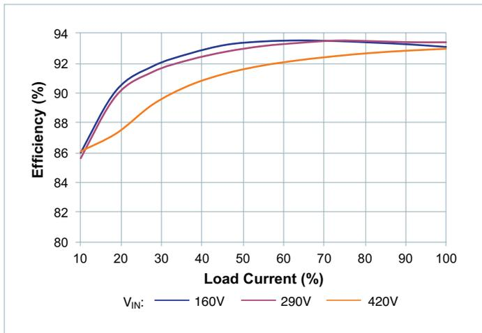
Figure 11 —  $V_{IN}$  to  $V_{OUT}$  efficiency,  $T_{CASE} = 90^\circ\text{C}$
