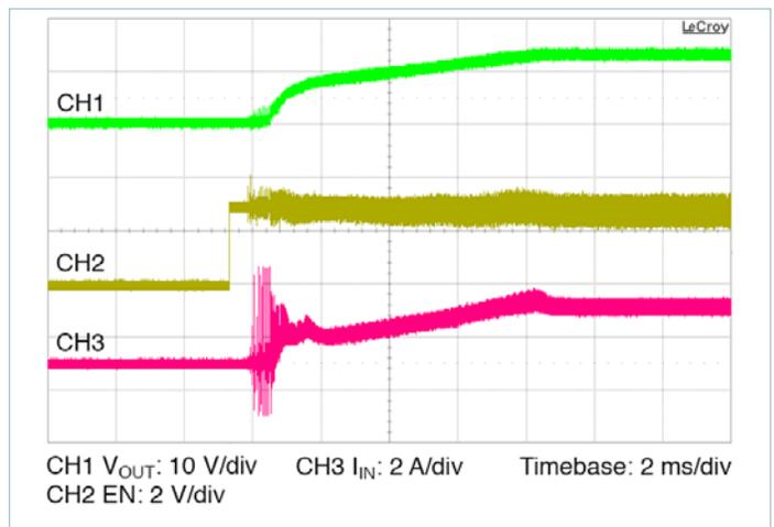
Figure 6 — Initial start up from EN pin, with soft-start ramp.
