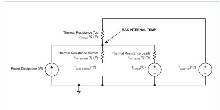
**Figure 23 — One-side cooling and leads thermal model**
