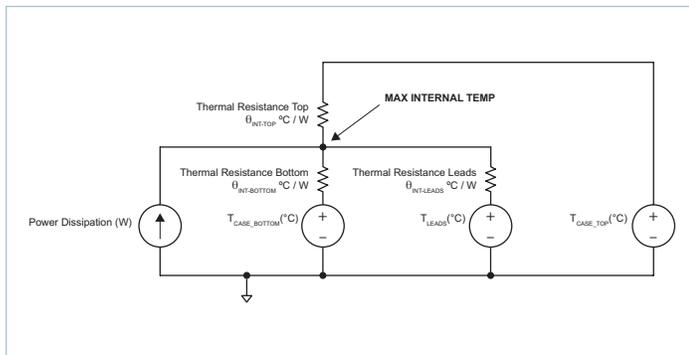
**Figure 22 — Double-side cooling and leads thermal model**
