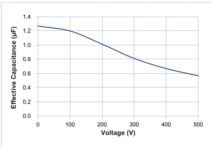
Figure 18 — Effective internal input capacitance vs. applied voltage
