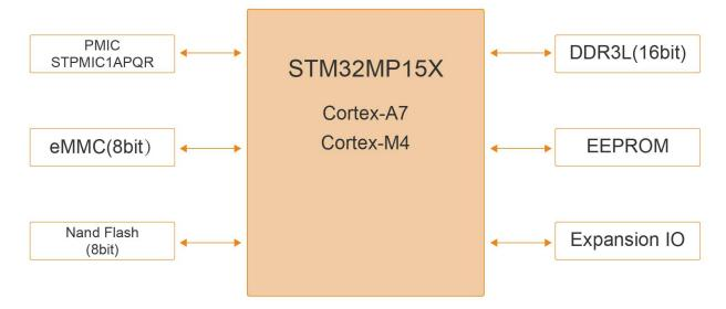
MYC-YA15XC-T CPU Module Function Block Diagram
