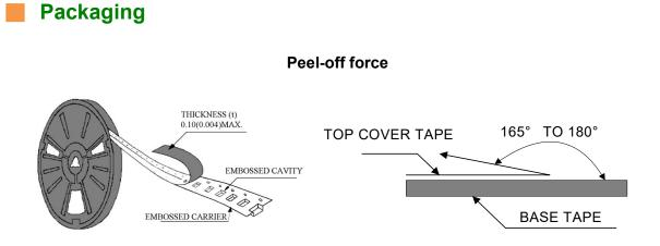
The peel off force of cover tape is 10 to 130 grams in the arrow direction.
