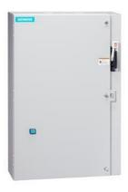
Non-reversing motor starter, Size 2 1/2, Three phase full voltage, Solidstate overload relay, OLR amp range 25-100A, Combination type, 100A fusible disconnect, 100A/600V fuse clip, Enclosure NEMA type 1, Indoor general purpose use, Extra-wide enclosure
