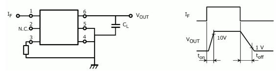
Fig. 11.1 Switching Time Test Circuit, Waveform
