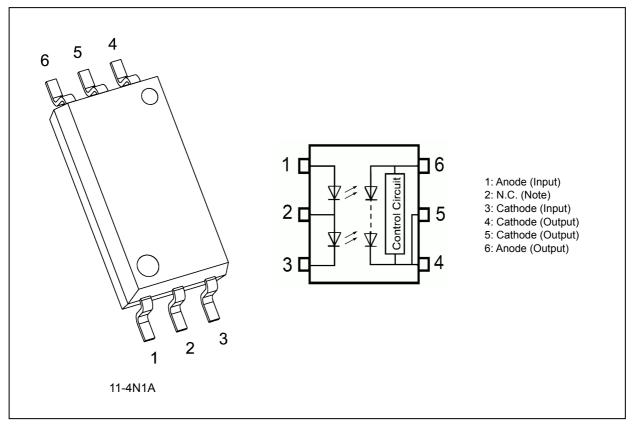
Note: Input side is considerd 2 LEDs serial connection.(i.e. Foward mean pin 1 to 3, Reverse mean pin 3 to 1.) Don't connect anything to pin 2.
