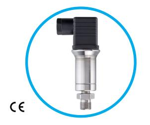
The external mount hydrostatic level transmitter, ILSE, has a piezoresistive silicon pressure sensor which is an oil filled isolated diaphragm. The sensor and housing are made from stainless steel with a choice of internal O ring seals to ensure the product is suitable for a wide range of applications.
