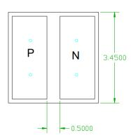
Figure 2. IN-C35PUDTDU1 Package Dimension
