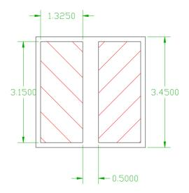
Figure 1. IN-C35PUDTDU1 Recommended Solder Pattern
