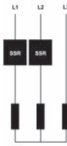
Two-phase SSR SOB to control heaters connected in star (for balanced low voltage loads without neutral connection)
