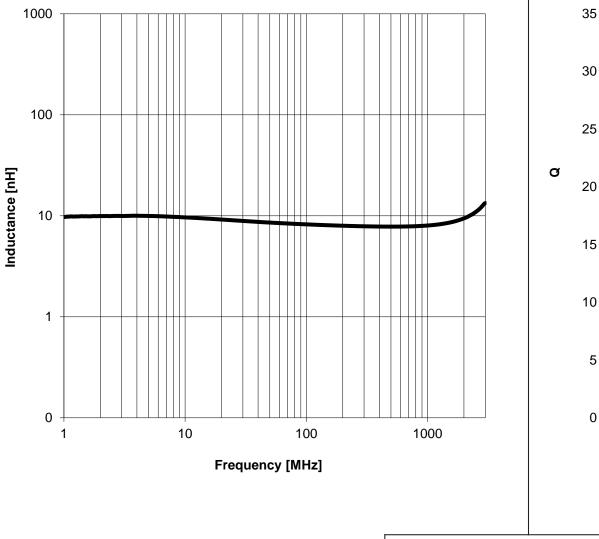
Typical Inductance vs. Frequency Characteristics:
