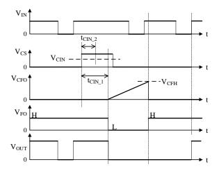
Figure 10-5. Overcurrent Protection Operational Waveforms 1
