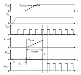
Figure 10-2. Startup Waveforms 1
