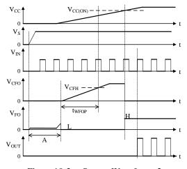
Figure 10-3. Startup Waveforms 2
