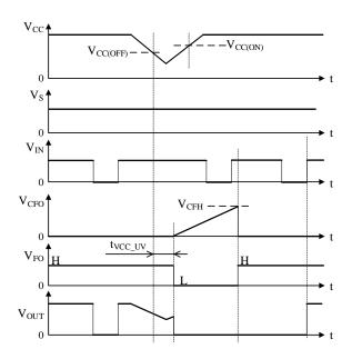
Figure 10-4. Undervoltage Lockout for Power Supply Operational Waveforms
