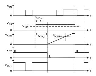
Figure 10-6. Overcurrent Protection Operational Waveforms 2
