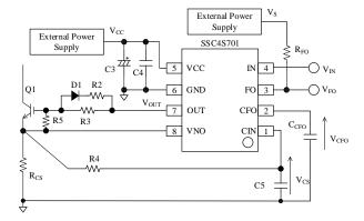
Figure 10-1. SSC4S701 Peripheral Circuit
