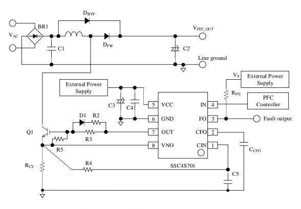
Figure 7-1. PFC Circuit Example Using SSC4S701
