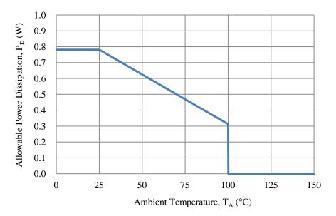
Figure 4-1. Thermal Derating Curve
