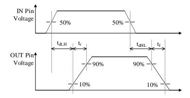
Figure 3-2. Input and Output Waveforms
