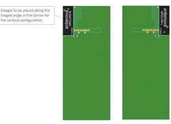
Vertical placement optimal minimum GND length required is ≥100mm
