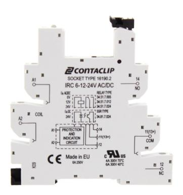
Interface-Relay-Compact (IRC) socket base IRC with screw connection, Mounting type: Mounting rail TS 35, 1 CO contact, Input voltage: 6, 12 or 24 VAC/DC
