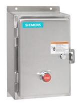
Non-reversing motor starter, Size 1, Three phase full voltage, Solid-state overload relay, OLR amp range 10-40A, Non-combination type, Encl. type 4X 304 S. Steel, Water/dust tight noncorrosive, Standard width enclosure
