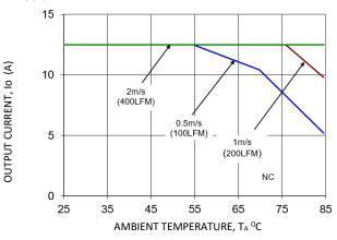
Figure 2. Derating Output Current versus Ambient Temperature and Airflow. Data shown for 115VAC in, at 230VAC in derating is the same or better. For derating at other input voltages, consult the GE Technical representative.
