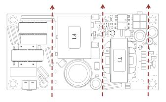
Fig. 10. Preferred airflow direction for cooling.
