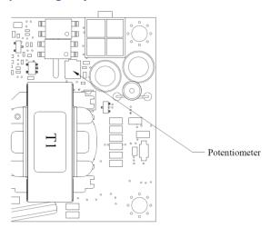
Fig. 9. Diagram showing location of the potentiometer used to adjust the power supply output voltage.
