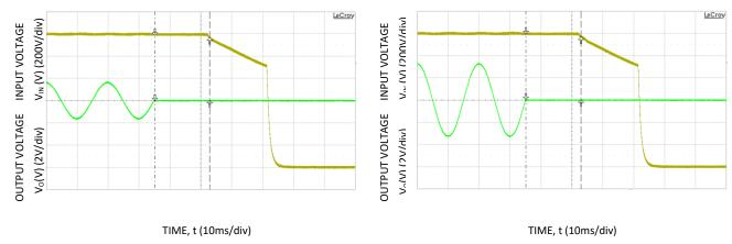
Figure 7. Typical Hold-up waveforms (Vin = 115V, 100% load).
