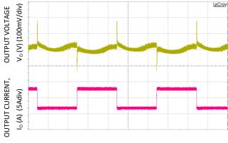
Figure 4. Transient Response to Dynamic Load Change from 50% to 100% at Vin = 230Vac.
