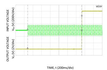
Figure 5. Typical Start-up (VIN = 115Vac).
