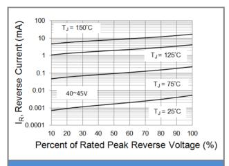
Fig.3 Typical Reverse Characteristics
