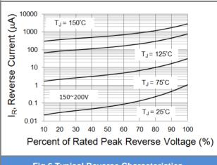
**Fig.6 Typical Reverse Characteristics**
