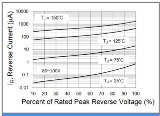
**Fig.5 Typical Reverse Characteristics**
