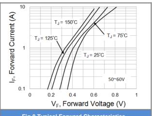
**Fig.8 Typical Forward Characteristics**
