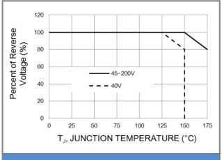
**Fig.11 Operating Temperature Derating Curve**
