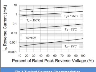
**Fig.4 Typical Reverse Characteristics**
