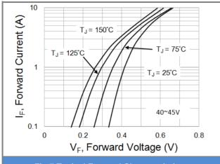
**Fig.7 Typical Forward Characteristics**
