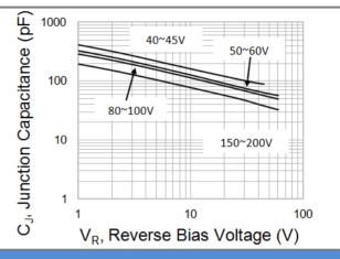
Fig.2 Typical Junction Capacitance
