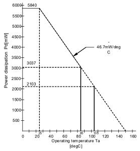
Figure 7-1. Thermal Derating characteristic
