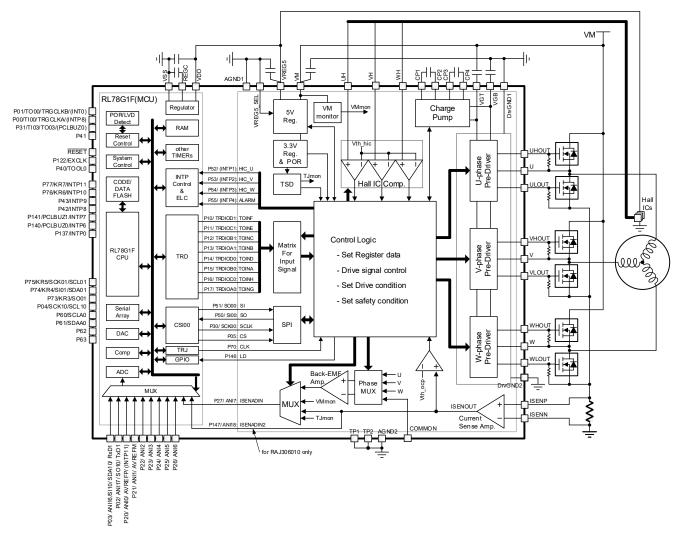
Figure 4-1. Block Diagram (Hall IC type)
