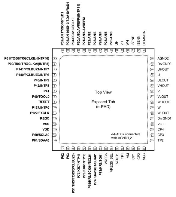
Figure 5-1. Pin configuration diagram
