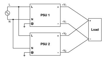
Fig. 4 Parallel Operation Connection Diagram
