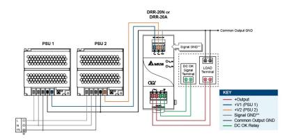
Fig. 3 Redundancy Operation Connection Diagram
