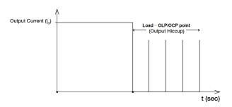
It is not recommended to prolong the duration of  $l_0$  when it is less than OLP/OCP point, but greater than 100%, since it may cause damage to the PSU.
