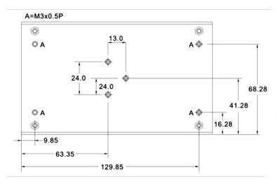
Customer is advised to screw into the threads no more than 1.5mm
