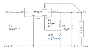
The values of R1 [adjust up], and (R2) [adjust down], can also be calculated using the following formulae.
