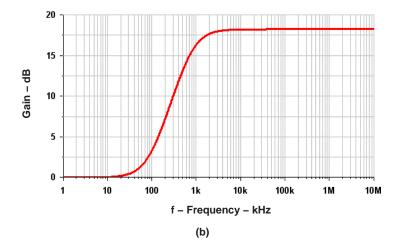
Note that the high pass filter function is not a true high pass filter. C3 in series with R7 creates a zero at about 10 Hz. As the frequency decreases from about 3 kHz to 10 Hz, the circuit changes from a gain stage into two unity gain buffers.
