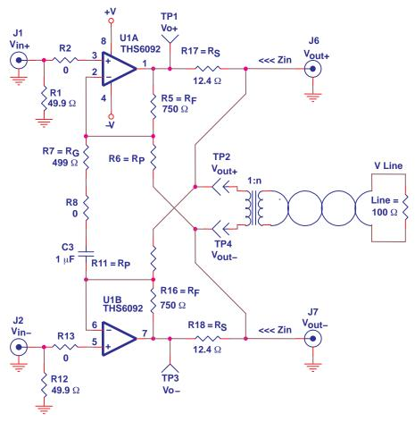
Active feedback creates larger impedance (Z) than what is actually placed there by series resistors R<sub>S</sub>:
