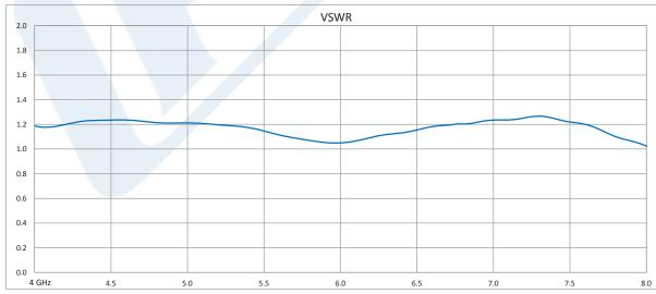
Click the following link (or enter part number in "SEARCH" on website) to obtain additional part information including price, inventory and certifications: Dual Junction Circulator With 36 dB Isolation From 4 GHz to 8 GHz, 10 Watts And SMA Female PE83CR1019
