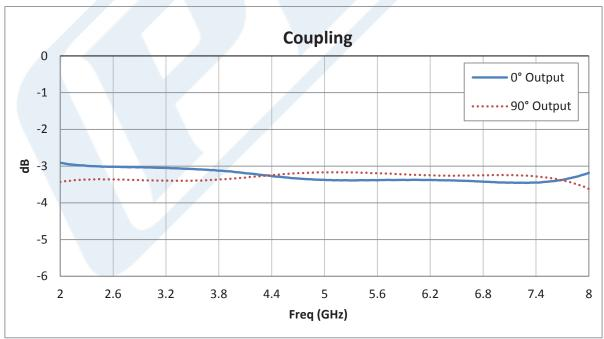
Click the following link (or enter part number in "SEARCH" on website) to obtain additional part information including price, inventory and certifications: 90 Degree SMA Hybrid Coupler From 2 GHz to 8 GHz Rated to 30 Watts PE2058
