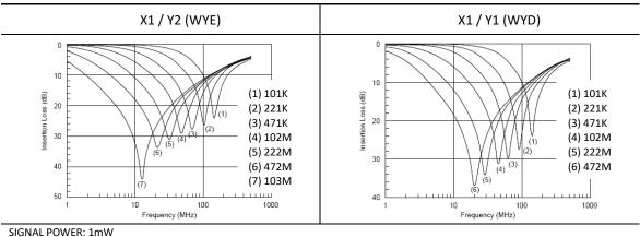
AC240V (R.M.S.) / 60HZ IS APPLIED ON THE CAPACITOR
