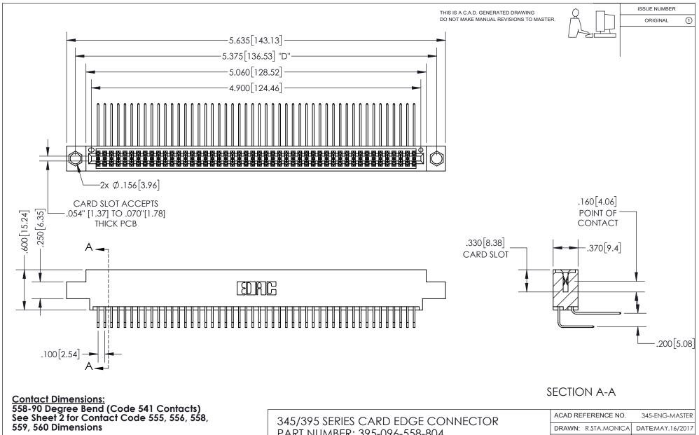
INSULATOR MATERIAL: THERMOPLASTIC PBT, UL 94V-0 CONTACT MATERIAL; COPPER TIN ALLOY CONTACT PLATING: GOLD ON THE MATING AREA, TIN PLATING ON THE CONTACT TAILS, NICKEL UNDERPLATE
