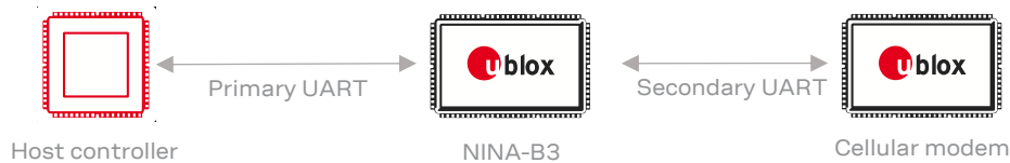
Figure 3: Example use case of the secondary UART interface
