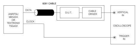
Fig. 2 Test Set-up 1
