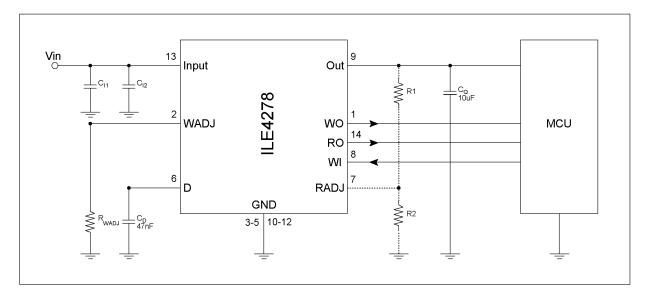
Figure 3. Typical application circuit
