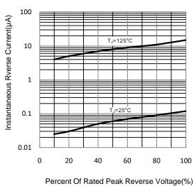
Fig.4 Typical Reverse Characteristics
