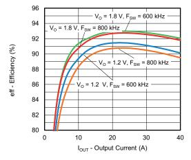
Fig. 1 - Efficiency vs. Output Current (V<sub>IN</sub> = 12 V, L = 100 nH, V<sub>CC</sub> = V<sub>DRV</sub> = 5 V)
