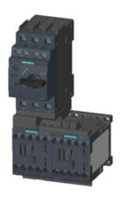
Fuseless motor starter Reversing operation 600VAC Size S00 1.4-2A 24V DC screw connection For screw mounting Or 35 mm rail-mounting Type of coordination 2 IQ = 150 KA Also full fills type Of coordination 1 1NO+1NC (MSP) 1NC (per contactor)
