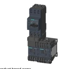
Load feeder fuseless, reversing duty 400 V DC, size S00 0.90...1.25 A, 24 V DC Spring-type terminal for installation on standard mounting rail (also fulfills type of coordination 1) Type of coordination 2, Iq = 150 kA 1 NC (contactor)
