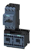
Fuseless motor starter Reversing operation 600VAC Size S00 0.11-0.16a 24V DC screw connection For screw mounting Or 35 mm rail-mounting Type of coordination 2 IQ = 150 KA Also full fills type Of coordination 1 1NC (per contactor)
