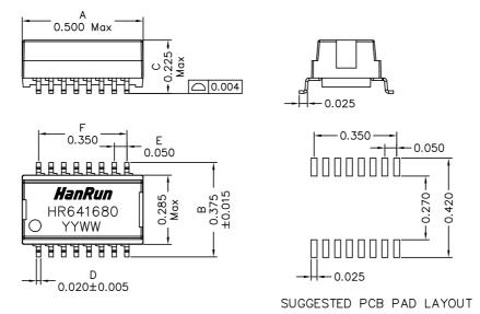
Dimensions in inches Unless otherwise specified, Tolerance: .xxx  $\pm 0.010$  REV.: 00
