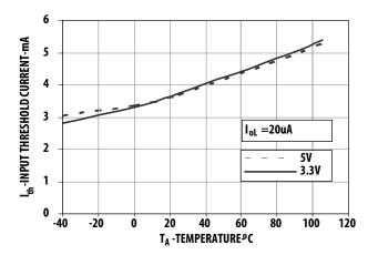
Figure 2. Typical input threshold current vs. temperature.
