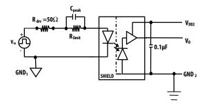
Figure 10. Connection of peaking capacitor (Cpeak) in parallel of the input limiting resistor (Rllimit) to improve speed performance
