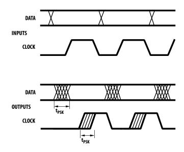
Figure 9. Parallel data transmission example
