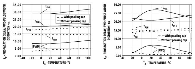
(i) V<sub>DD</sub>=3.3V, C<sub>peak</sub>=100pF, R<sub>limit</sub>=80Ω
