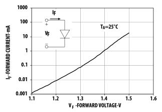
Figure 1. Typical input diode forward characteristic.
