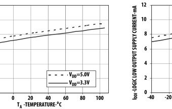
Figure 3. Typical logic high 0/P supply current vs. temperature for QCPL-074H.
