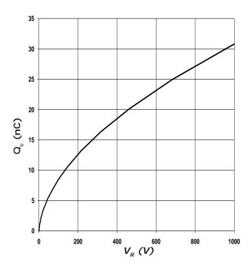
Figure 5. Recovery Charge vs. Reverse Voltage
