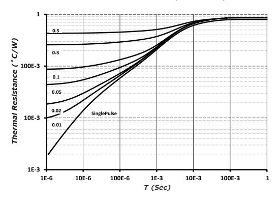
Figure 9. Device Transient Thermal Impedance
