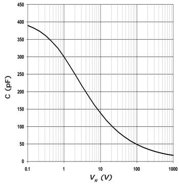
Figure 6. Capacitance vs. Reverse Voltage
