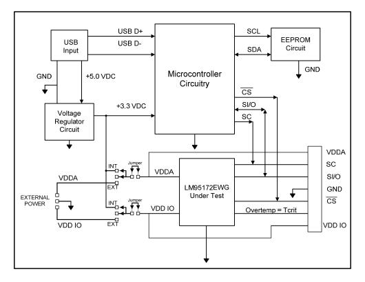
Figure 3: LM95172EVM Block Diagram
