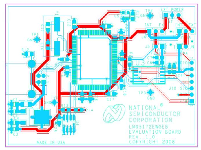
Figure 5: LM95172EVM Layout Diagram
