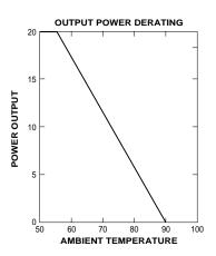
Typical Performance: (Tc=25°C, Vin=Nom VDC, Rated Load)
